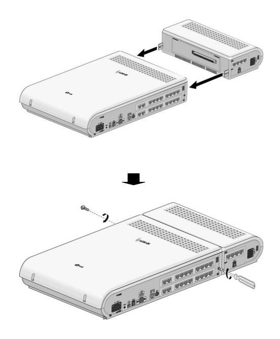
Figure 4.3.1 Connecting an expansion module
